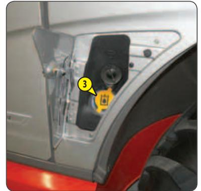
**REPLACING THE HYDRAULIC RETURN OIL FILTER CARTRIDGE**
